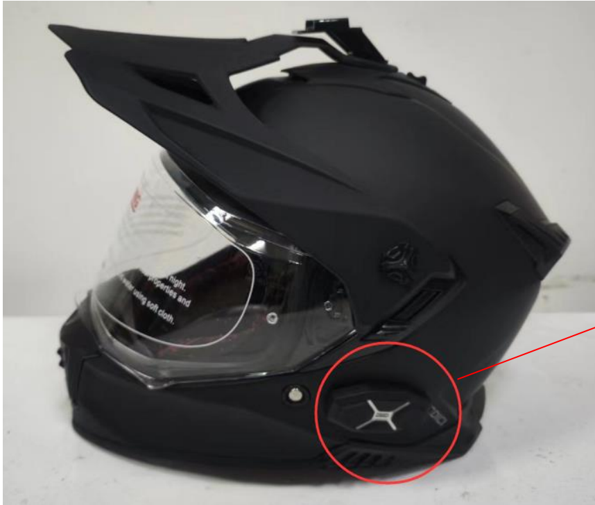
1 - Way of fixation: attached to helmet by screws
