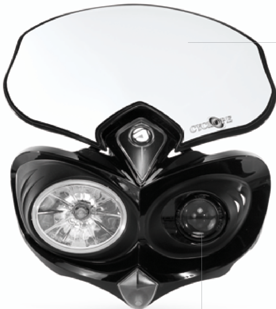
Faro con lampadina alogena da 55w Light beam with 55w alogen bulb
